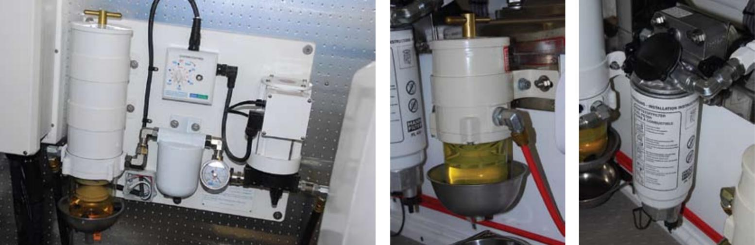
ESI fuel polishing system can polish fuel from any of the four tanks. (top left) Generator primary fuel filters use highly-effective Racor Turbine design. (top center) Additional engine primary filter provides triple filtration. (top right) High-volume fuel transfer pump can move fuel between any two tanks. (bottom)
